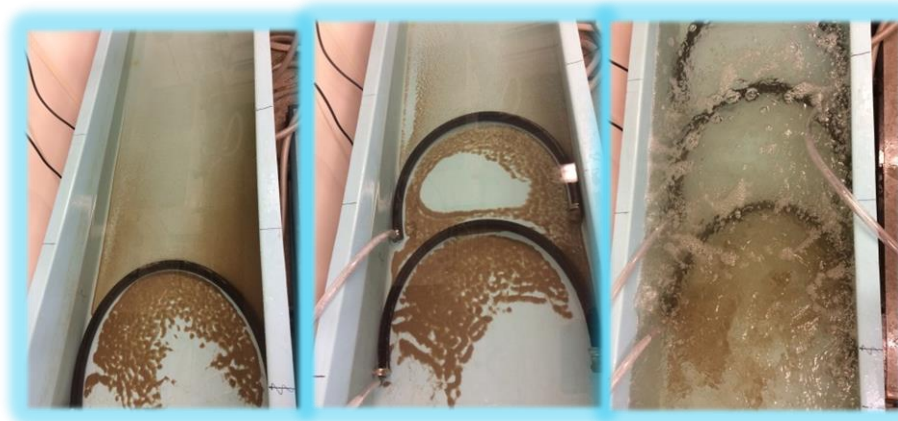
Figure 8: Settled very-fine sand (125-63 \mu\text{m} ) with one, two and three Bubble Tubing ® layers.
