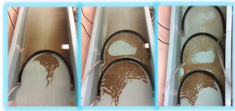
Figure 7: Settled fine sand (250-125 \mu\text{m} ) with one, two and three Bubble Tubing ® layers.
