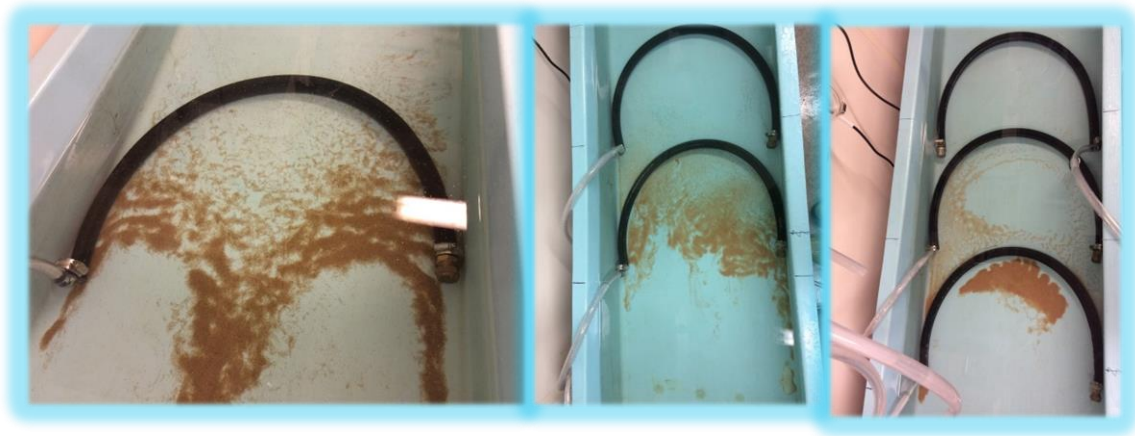
Figure 6: Settled medium sand (500-250 \mu\text{m} ) with one, two and three Bubble Tubing ® layers.
